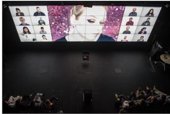
**Figure 2:** The CALIT2 VROOM features a tiled display of 32 full HD narrow-bezel screens that can be employed distinctly, or as a single surface, yielding up to 66 million pixels on the entire wall (15,360 x 4,320 pixels).
